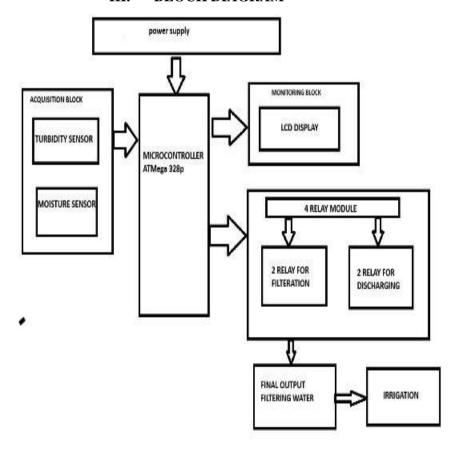
The researchers created the block diagram that would act as the system's architecture and is displayed in Figure 3 to show how the Microcontroller Based Wastewater Management System functions. The system's primary component is the microcontroller. It controls the entire process in some way.
